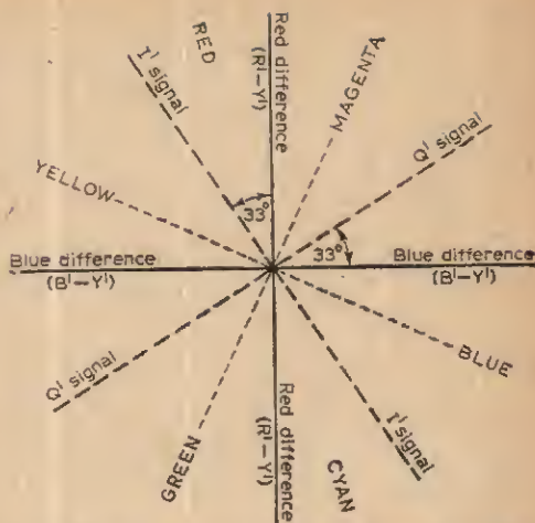
Fig. 25—Colour vector diagram. The I' and Q' signals differ in phase from the associated red and blue difference-signals by 33 deg.
